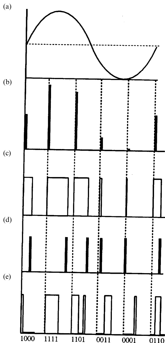
Figure 1. Four different digital versions of the same simple analogue signal (a). For the sake of clarity these diagrams are coded with only 4 bits (normally 14, 16 or more bits are used), and show only a small proportion of the hundreds or thousands of sample 'slices'. A sequence of measurements of an analogue signal requires values both for time (horizontal axis) and for amplitude (vertical axis). All measurements of a digital signal are related to a constant, very short time unit, so that only one value is needed: these diagrams show the signal depicted by pulse amplitude (b), width (c), time displacement (d) and, the simplest, its coded binary numerical value (pulse code) (e). The dotted line in (a) is a representation of the zero amplitude axis normally used to show the positive and negative values of an analogue signal. In all diagrams of figure 1 this zero line has been lowered so that the base line is now zero. This avoids the use of complex coding systems to represent negative numbers.
